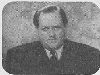
2. Effect of setting brightness control too low
