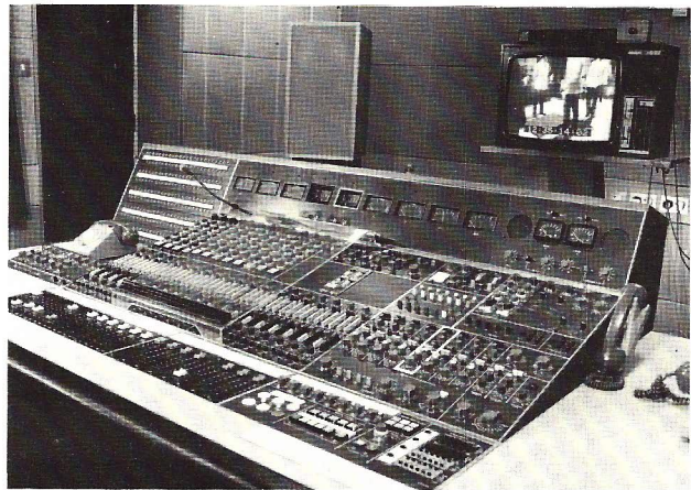
Fig. 5 Sound control desk and picture monitor showing inset time-code.
