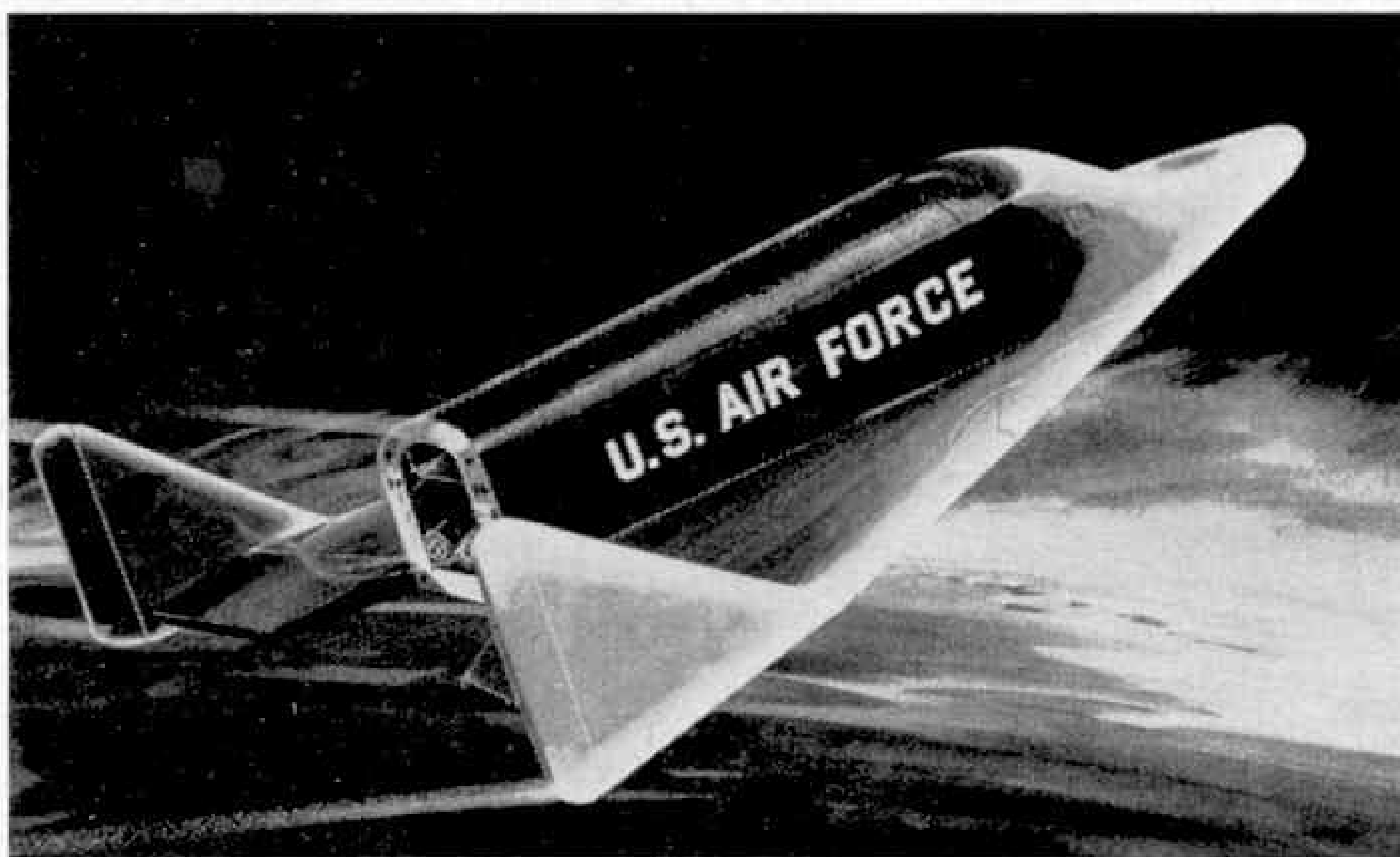
As the Dyna-Soar re-enters the Earth's atmosphere after a flight into space, its leading edges will glow from the heat created by the friction of the glider passing into the atmosphere.
