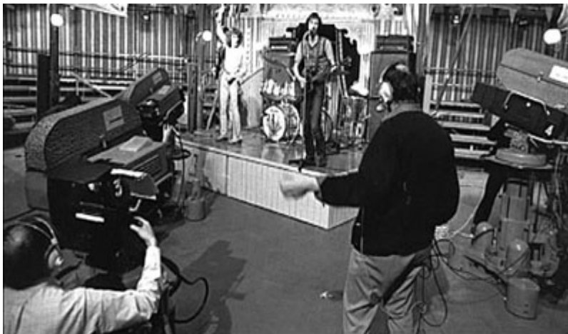
This still of The Who shows the French hybrid TV/16mm film cameras hired in to make the Rolling Stones Rock and Roll Circus . The cameramen are framing using a video CRT viewfinder. However, on the top of each camera is a magazine for film reels. The image was split and passed to the video camera to enable the shot to be previewed and also to a film camera enabling the image to be recorded. Thus the show could be directed using multicamera TV methods but the final print would be on colour film and capable of being shown anywhere in the world.
