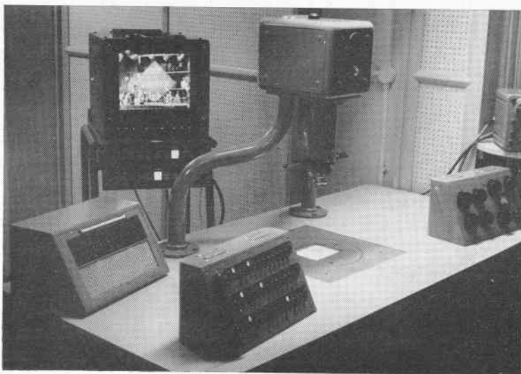
Inlay/Overlay equipment for the production of special effects. An example of its use is illustrated. A portion of the picture from one camera is blacked out by placing a diamond shaped mask over the raster from a flying spot scanner in the centre of the control desk. This space is filled with a caption from a second camera.
