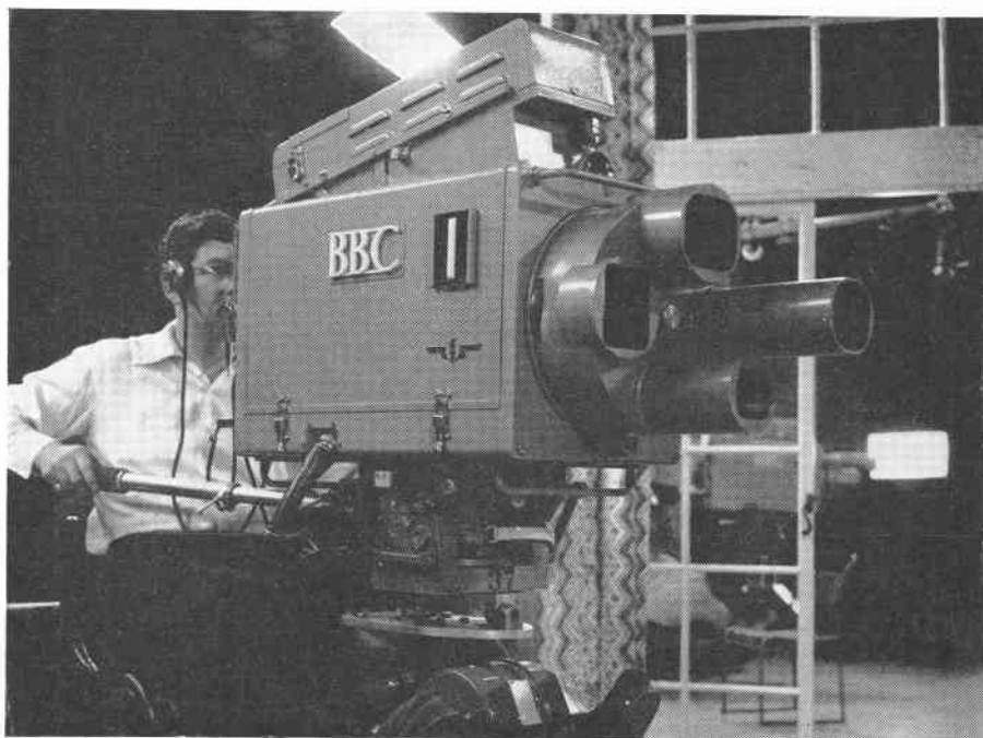
One type of modern camera showing the rotating lens turret, fitted with four lenses of different focal lengths, and an electronic viewfinder.
