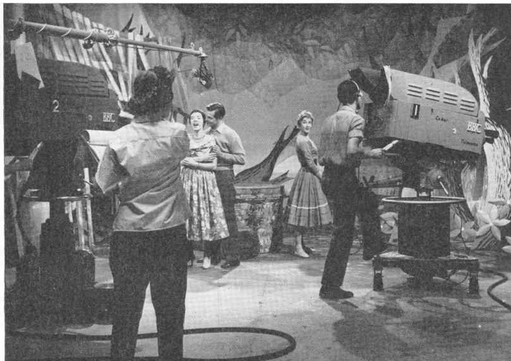
BBC Experimental Colour Television transmissions. A view of the studio at Alexandra Palace showing the two three-tube colour cameras.
