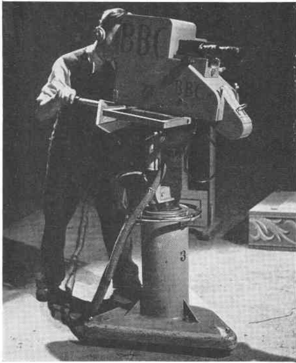
An example of a pre-war camera fitted with a single lens and optical viewfinder.
