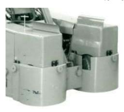
In studio use, the cable guards were dropped as near to the studio floor as possible, to allow the crane to push away all types of cables – including mains cables and (in particular) microphone cables: there were all sorts of cables trailing around a studio floor! With the bottom of the guards near to the floor, it was near impossible to see the Heron wheels from the outside.
